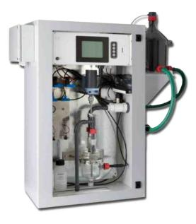
The DIMA-CenoTOX<sup>®</sup> is an online analyser for toxicity determination. It evaluates oxygen consumption and differentiates nitrification, carbon oxidation and sulfur oxidation. The DIMA-CenoTOX<sup>®</sup> allows the rapid detection of harmful wastewater streams and enables you to react quickly when the biology is in danger.
