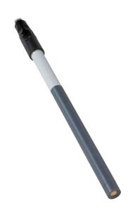
Ion-selective electrode for nitrate with replaceable membrane head.
