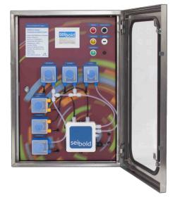
The online analyser "Heinrich Proch" from Seibold's Composer analyser family continuously determines the chromium concentration. It is suitable for monitoring of toxic, carcinogenic chromium(VI) as well as for total chromium.
