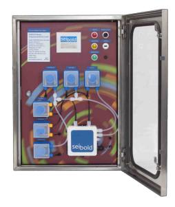
The online analyser "Franz von Suppé" from Seibold's Composer analyser family continuously determines the aluminium concentration.
