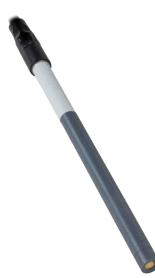
Ion-selective electrode for nitrate with replaceable membrane head.
